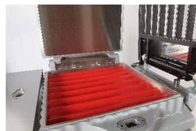
Robotrad-s Form : Moulding dividers with side grill and forming plate.
