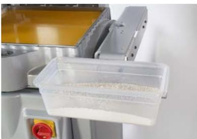
Handy removable flour tray with top cover which can be fixed on various positions on the machine.
