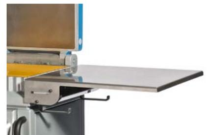
Stainless steel working table on left or right side which can be folded down completely.
