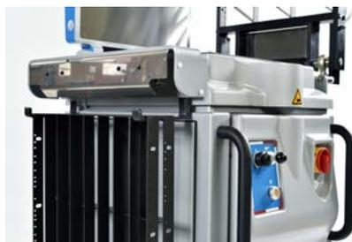
Storage hooks for max. up to 6 grids on one or both sides of the machine.
