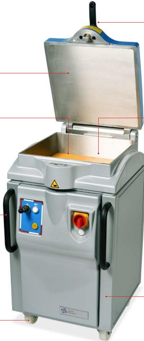
Solidly constructed grip and locking mechanism for opening and closing of the lid in one fluent natural movement.
