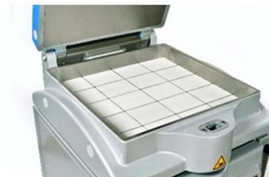
Dividing disc made out of easy exchangeable food grade ertalyte dividing segments.
